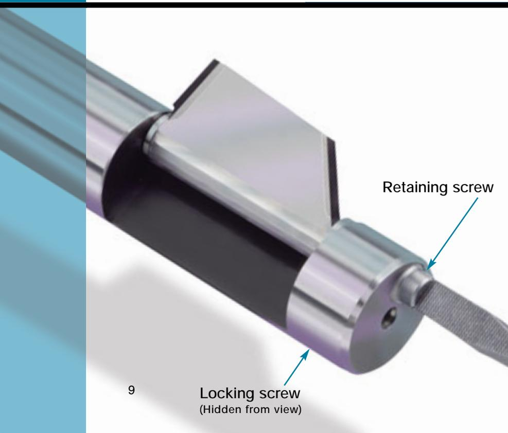
To ensure that the cutter rotates freely in the arbor, with no end float, adjust the retaining screw until the cutter binds, then back off approximately 5 degrees. Use the locking screw to lock the retaining screw at this position.
