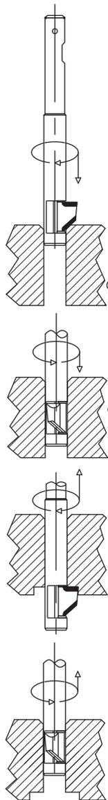
1. The front chamfer is machined upon entry into the bore, using right hand rotation (clockwise) of the machine spindle at the appropriate speed (refer to chart on page 10), and .002 IPR (0.05mm/rev).
